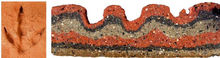
Figure 1. Vertical section through emu track emplaced in package of layered cement revealing the formation of undertracks in the layers subjacent to the true track.
